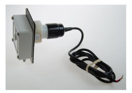
Properties Pump Housing: ABS Motor/Gearbox: Metal, Copper & Acetyl. Other Parts: PVC Spigots, Nylon Rollers, Stainless Steel bracket & pins. Mounting: Stainless Steel plate fitted with a Foam gasket. Peristaltic Tube: Santoprene Supply Voltage: 9V DC Running Current: 1.3A Capacity: Flow rate of 50 litres per hour using a 6.2mm bore Santoprene tube. Dimensions: 7.8 x 10.5 x 12 cm Net weight: 0.4 Kg Connection: Fitted with two core 1m cable.
