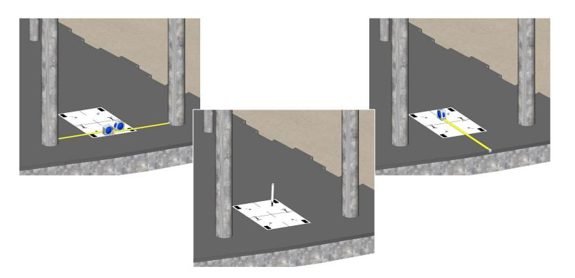
5. Remove the template, drill the holes through the matting and locate pronged T-nuts as per the instructions below. – If needed strike with hammer to ensure spikes grip into matting.
