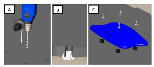
**A:** Drill correct diameter hole to correct depth.
