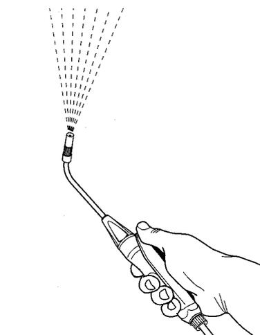
**IMPORTANT :** Purge air by spraying upwards with gun held above supply line.
