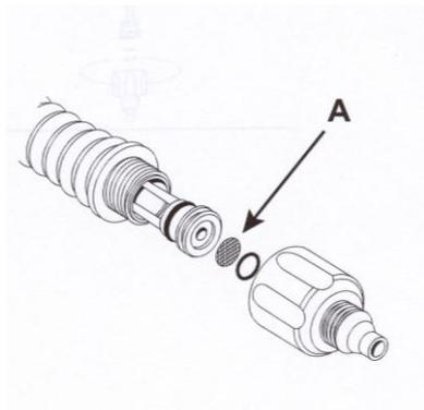
**IMPORTANT:** Nozzle is protected by filter (A). Should spray deteriorate or stop, remove and clean filter.
