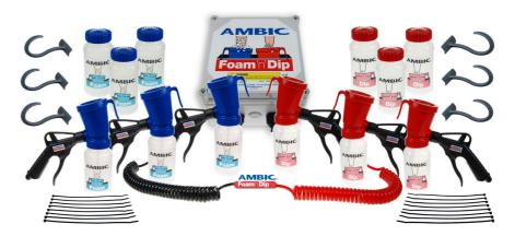
Foam'n'Dip™ is a simple, economical and yet highly effective dual purpose teat sanitisation system which generates low pressure compressed air to automate both pre- and post- teat sanitisation processes. The system comprises a mains operated dual purpose Air Power Unit which is used to operate a combination of Foam Applicators for pre-milking treatment and Dip Applicators for postmilking teat sanitisation.
