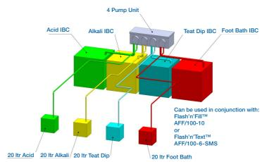
The Remote Delivery System™ is a microprocessor-controlled automatic / manual decanting system which can control the operation of up to four different Extra High Volume Peristaltic Pumps in order to refill header tanks containing fluids for cleaning or sanitisation purposes. Typical applications include the dispensing of acid, alkaline, footbath and teat sanitisation chemicals.
