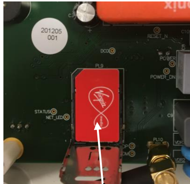
Place the SIM card face down
